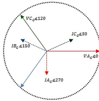
(a) Phase angle relationship between test source voltage and current in primary side of Transformer
