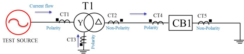
Fig. 1. Simplified Single-Line Diagram.
