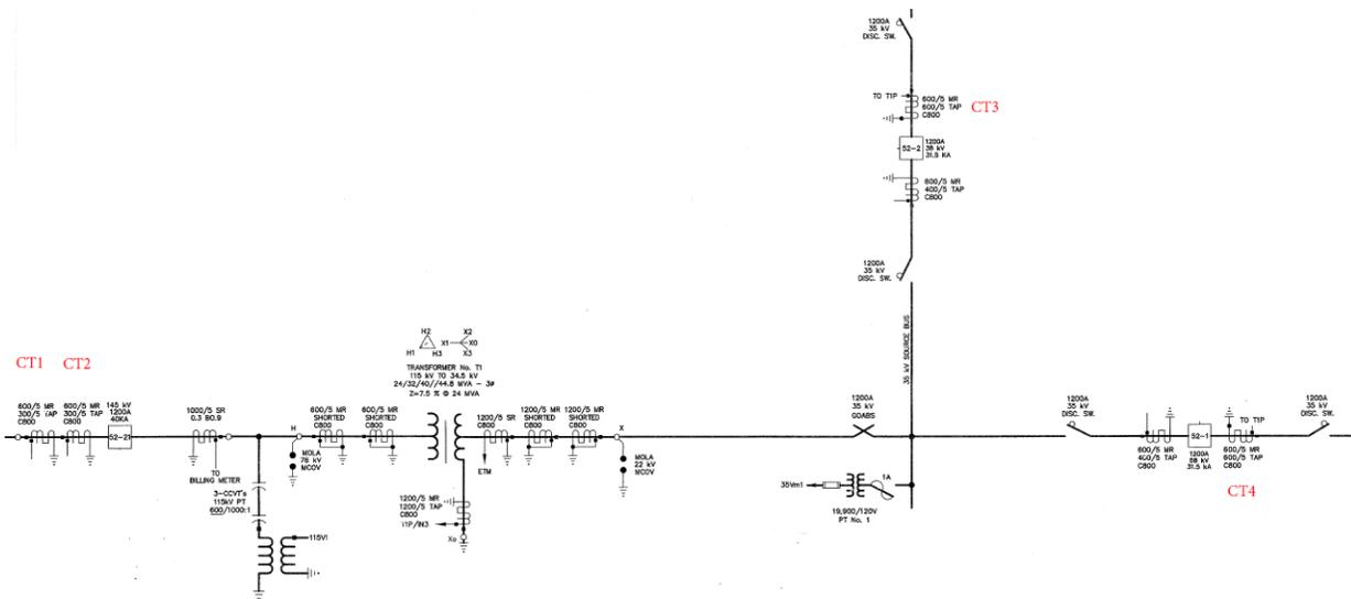
Fig. 3. Modified single line diagram of solar project.
