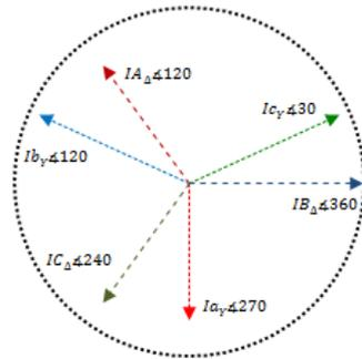
(b) Phase angle relationship between current in CT1 and CT2 seen by protective relay
